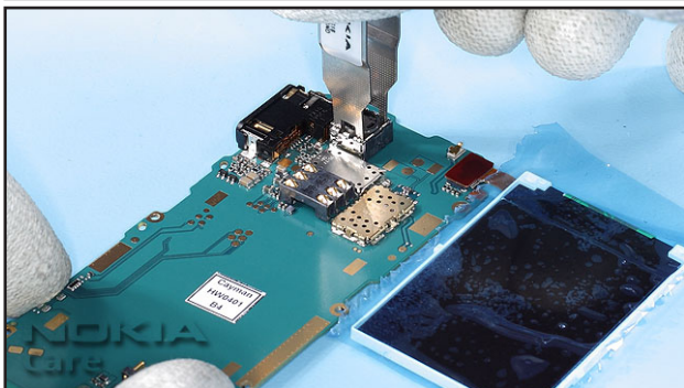
15. Flip over the LCD. Use the SS-88 for camera removal.
